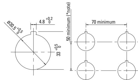
\*Note: The meter can be mounted on the top mounting holes of a standard 50mm mounting centers. The meter can be mounted on any mounting hole with a 70mm or larger mounting center.
