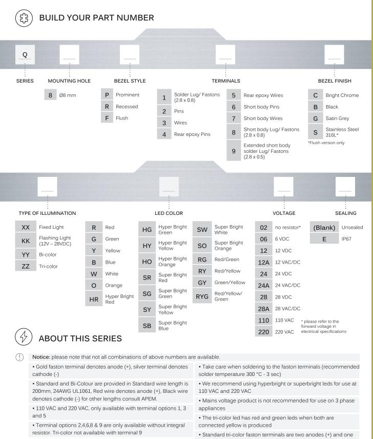
• Bi-color leds, by connecting the gold faston (+) one color is produced, by reversing the supply voltage another color is produced – bi-colors are available up to 28 VDC [AC products not available]
