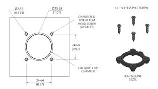
• The maximum panel thickness for the Rear Mount configuration is 2.032 mm (0.08 in).
