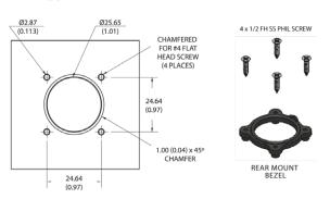
The maximum panel thickness for the Rear Mount configuration is 2.032 mm (0.08 in).
